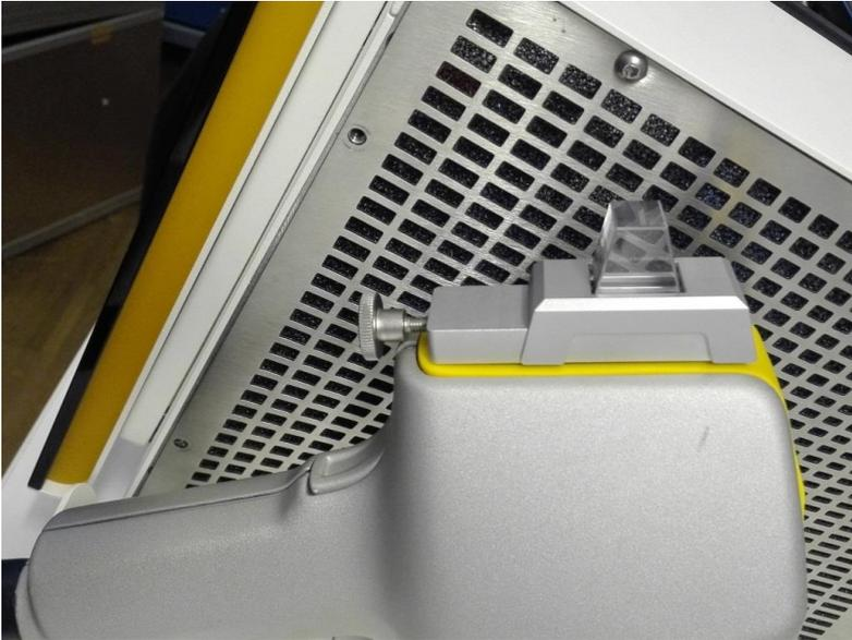
**Figure 5: Small spot adapter mounted on the sapphire crystal**
