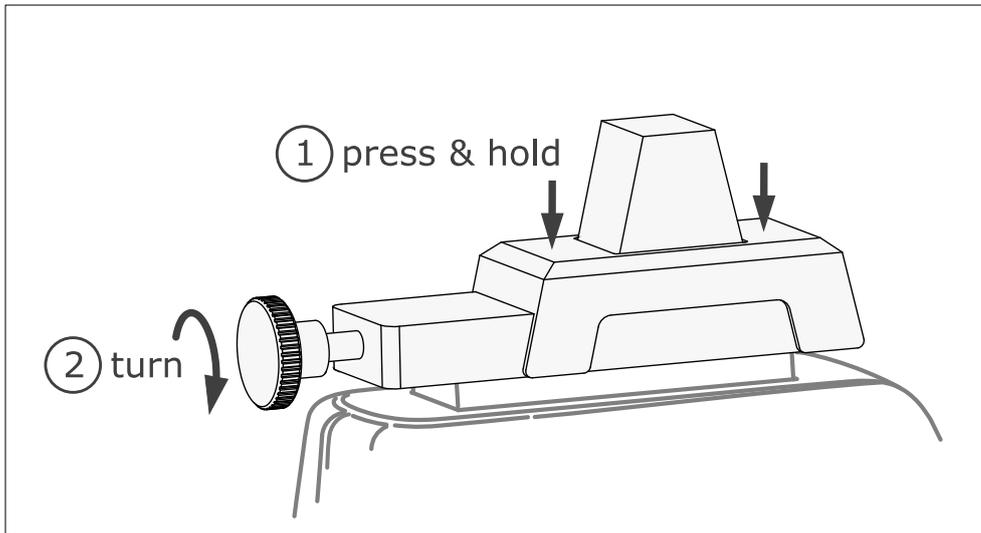
**Figure 7: Schematic drawing –fixing the small spot adapter**
